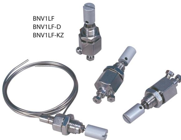
VICI regulators are machined from aluminum bar stock and then hard-anodized to provide contamination-free service. They feature a stainless steel diaphragm and Viton®-sealed stainless poppet. The compact size (1.125" diameter by 2" long for regulator, 3" long for combo version) saves panel space and permits installation anywhere that an 11/16" hole can be located. Mounting hardware is supplied.
