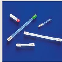
Release of the chemical occurs by permeation through the walls of the PTFE tube for the entire length between the impermeable plugs. A wide range of rates – typically from 5 ng/min to 50,000 ng/min – can be achieved by varying the length and thickness of the tube. These are the most widely used of the various permeation devices.
